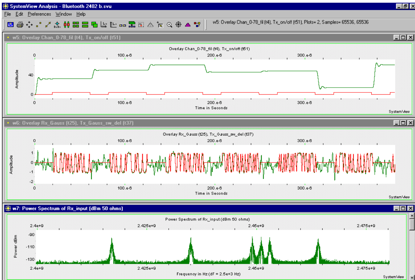
Figure 6. Path loss is 70 dB. (4,194,304 samples, 6.3 hops) (Fix Random Seed is set to 222.)
